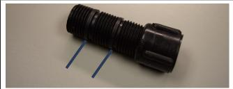
5. Gently unscrew the spray head from the funny pipe fitting or plastic nipple.
