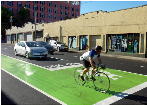
Above: Example of a bike box, where drivers must stop at the first white stop bar and a designated area at the head of a traffic lane provides bicyclists with a safe and visible way to get ahead of queuing traffic.
