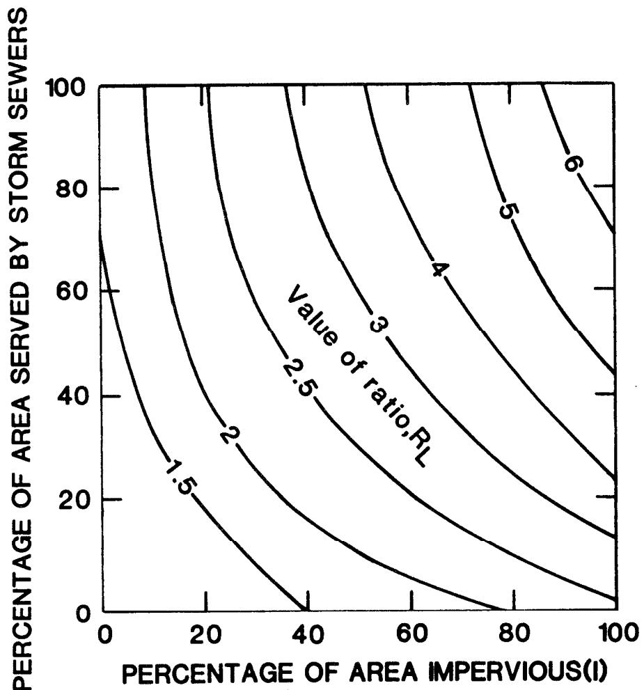
Figure 1.--The relationship of the urban adjustment factor,  $R_L$ , to the percentage of the area impervious and served by storm sewer. (Adapted from Leopold, 1968, by Sauer, 1971).
