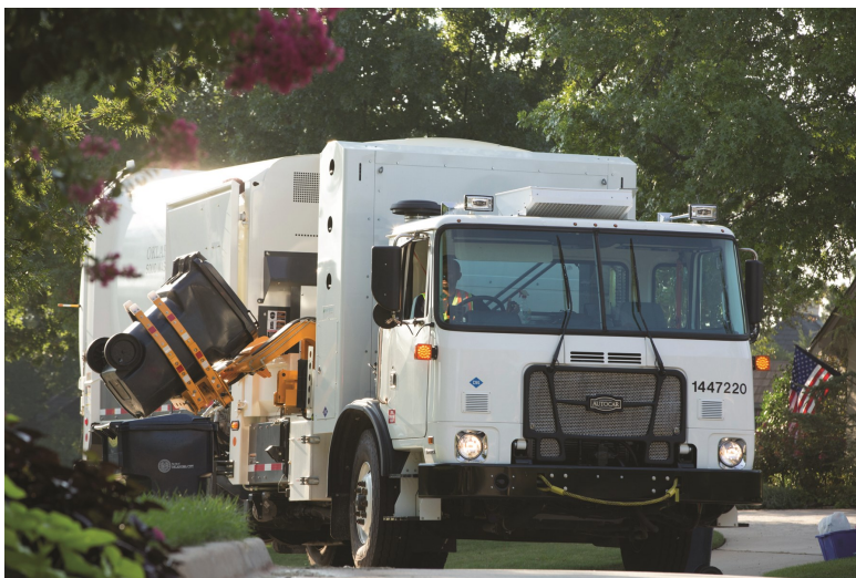
A semi-automated side loader trash truck empties customers' trash carts.
